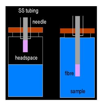
Fig 3. Adsorption phase in SPME extraction
